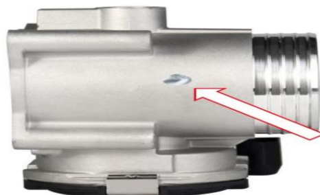
Figure 3. NG Dent on Throttle Body
