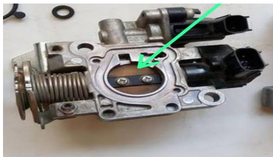
Figure 2. Throttle Valve On Throttle Body
