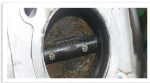
Figure 6. Rust on the Throttle Body
