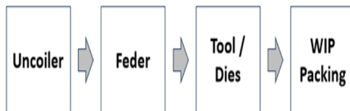
Figure 1. Stamping Process Block Diagram
