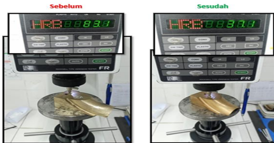
Figure 4 : Before and After Changing the Specification of Wiper Material Hardness
