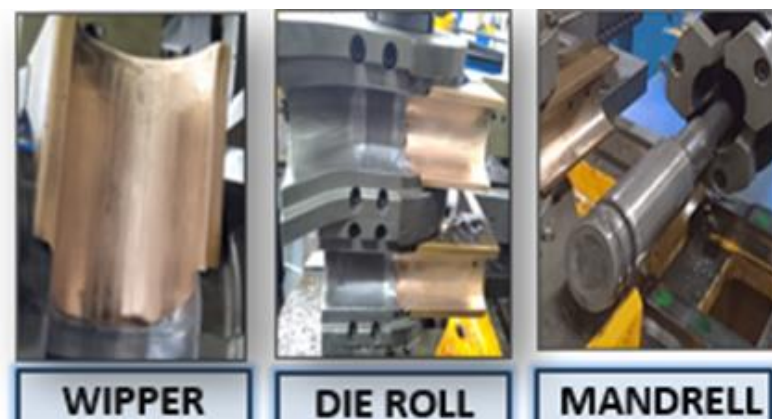
Figure 2. The mismatch of the radius of the wiper with the die roll, causes the part to wrinkle and corrugation.
