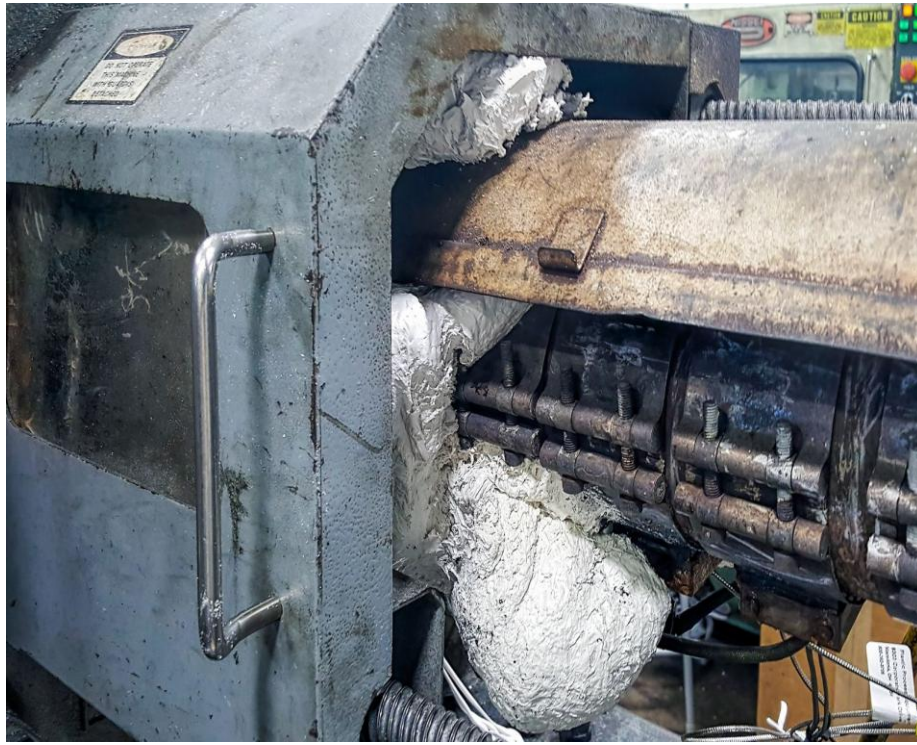
Figure 5. Polymer leakage in the injection molding machine
