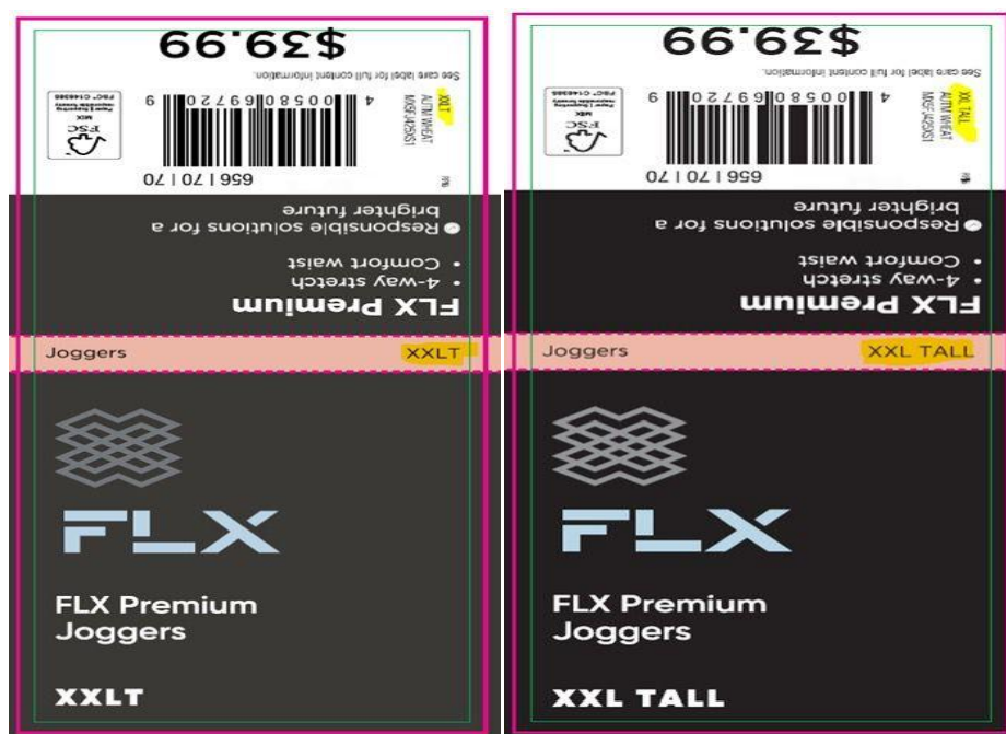
Figure 4. Mismatch of size format between layout and plate Source: Documentation of PT.XYZ (2025)
